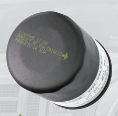
AMSOIL Oil Filters feature a reference arrow to aid in proper installation. Once the filter is finger tight, it is easy to gauge the additional .75 to 1.25 turns required to ensure a good fit. Over-tightening can lead to leakage.
